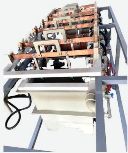
PTH CHEMICAL LINE
